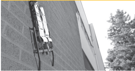
SRI's electroadhesive wall-climbing robot
