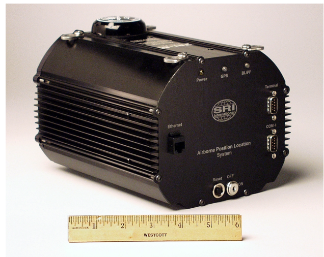
Figure 2. SRI airborne position and location system (APLS) GPS/IMU package (Strus et al. , 2002).
