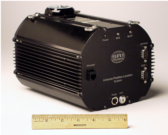
Figure 4. The APLS pallet instrumentation package.
