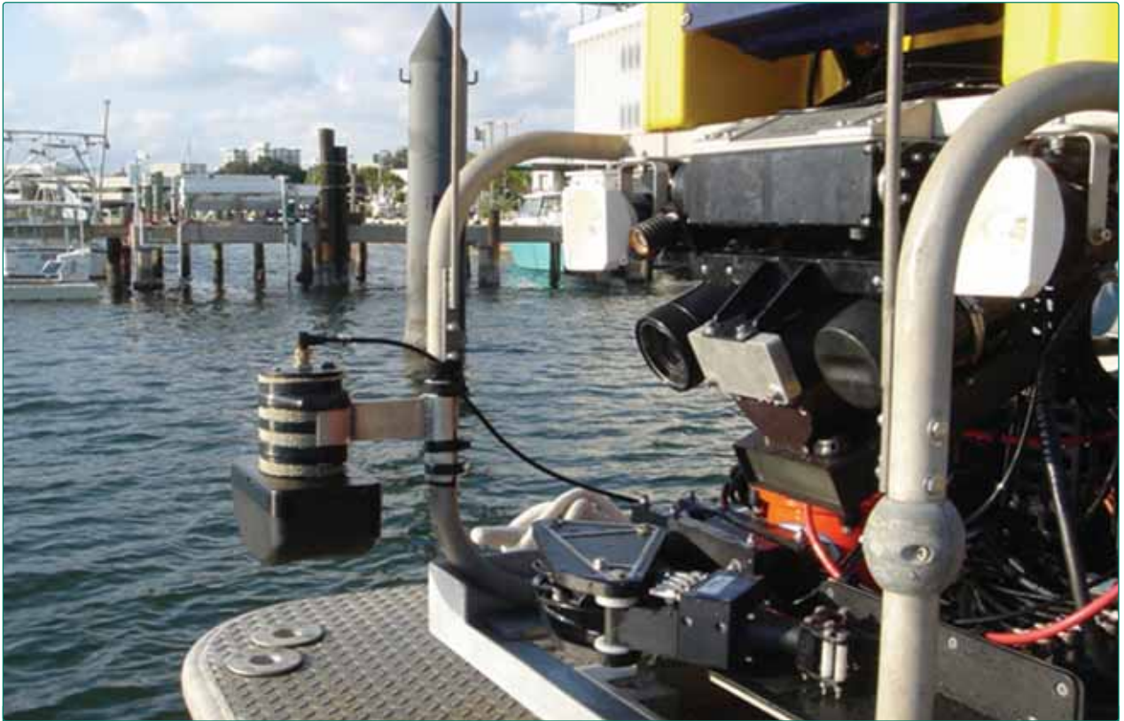
Remote operated vehicle for mine- or underwater-improvised explosive device detection.
