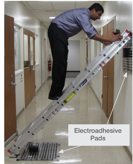
Traction enhancement application of electroadhesion to ladder safety
