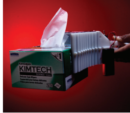
Application of electroadhesion to gripping complex-shaped objects
