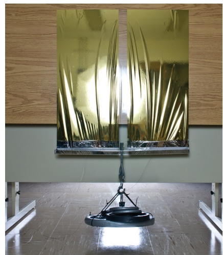
Electroadhesive pads on a wood surface supporting 75 lbs of weight
