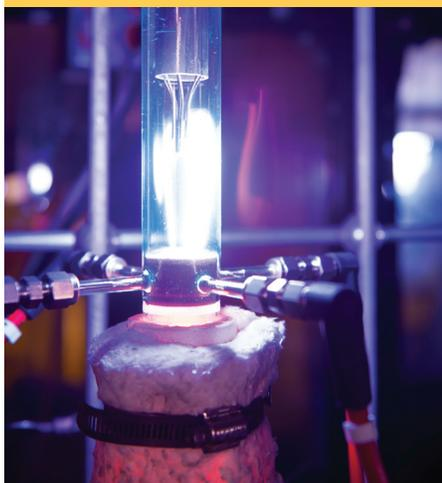
Operating 2-inch titanium granule multi-arc fluidized bed reactor
