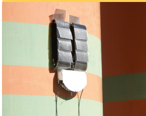
Electroadhesion-enabled wall-climbing inspection robot on industrial exhaust pipes
