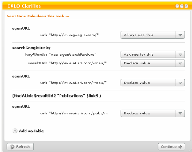
Figure 4. Clarification window for presenting a learned procedure and letting the user make adjustments to parameter settings.
