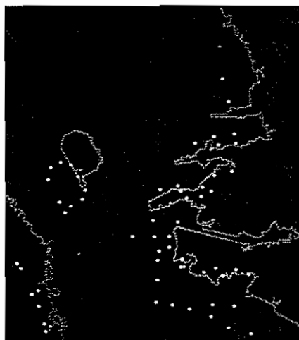
FIGURE 4 PREDICTED IMAGE COORDINATES OF COASTLINE, (BASED ON NAVIGATIONAL ESTIMATES OF CAMERA LOCATION AND ORIENTATION) SUPERIMPOSED ON EXTRACTED BOUNDARY
