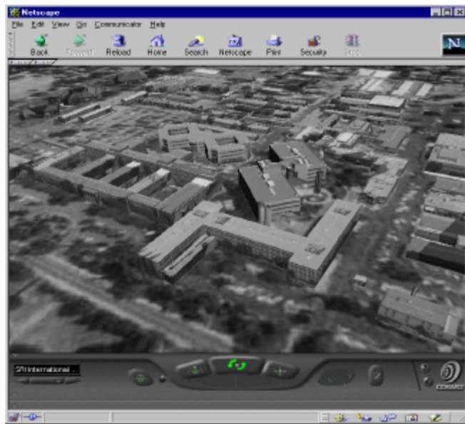
Figure 4. A texture-mapped site model of the SRI International campus that has been georeferenced onto an underlying terrain model. Note the accurate alignment of the latitude/longitude-specified buildings with the underlying 1 m resolution USGS DOQ satellite imagery in UTM coordinates.
