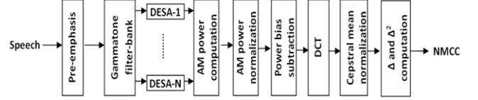
Figure 1: Flow-diagram of NMCC feature extraction from speech.
