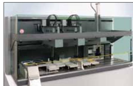
Figure 1: High Throughput Liquid Handling System.
