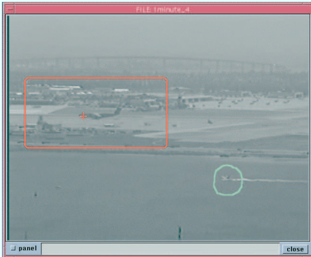
Figure 1. Video Player. Moving objects in surveillance regions are tracked (plane). Multimodal commands can target specific objects (boat).
