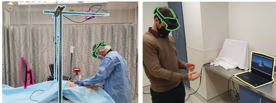
Local Server Camera mount Over-head RGBD camera Side-view RGBD camera Head-mounted display Remote Computer
