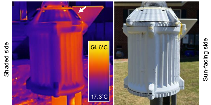
Thermal image of Finned-design. Note the painted sky-facing surface is colder than the shaded side.
