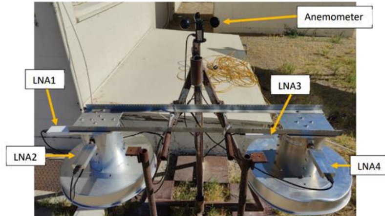
Test setup. Cylindrical parts are the feeds and the LNAs are mounted by coaxial connectors to the feeds.
