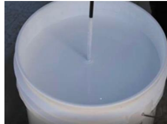
Paint was mixed in a 5-gallon container, without modification, using an overhead, open drum paint mixer.
