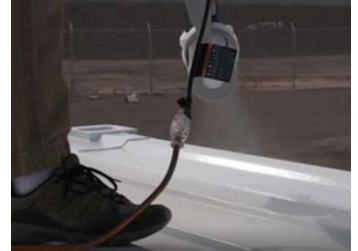
The paint was sprayed using a commercially available spray gun, without primer.
